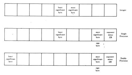
Figure D.3 Number Types in the Floating-Point Accumulator
