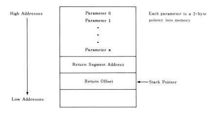
Figure D.1 Stack Layout When the CALL Statement Activated.
