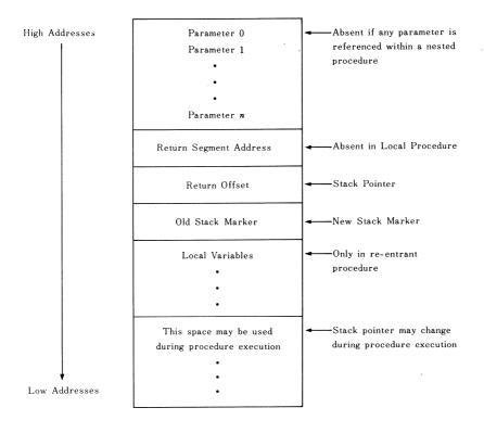
Figure D.2 Stack Layout During Execution of a CALL Statement.
